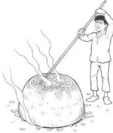
Fig.4. Pan roasting of cleaned cashew nut
